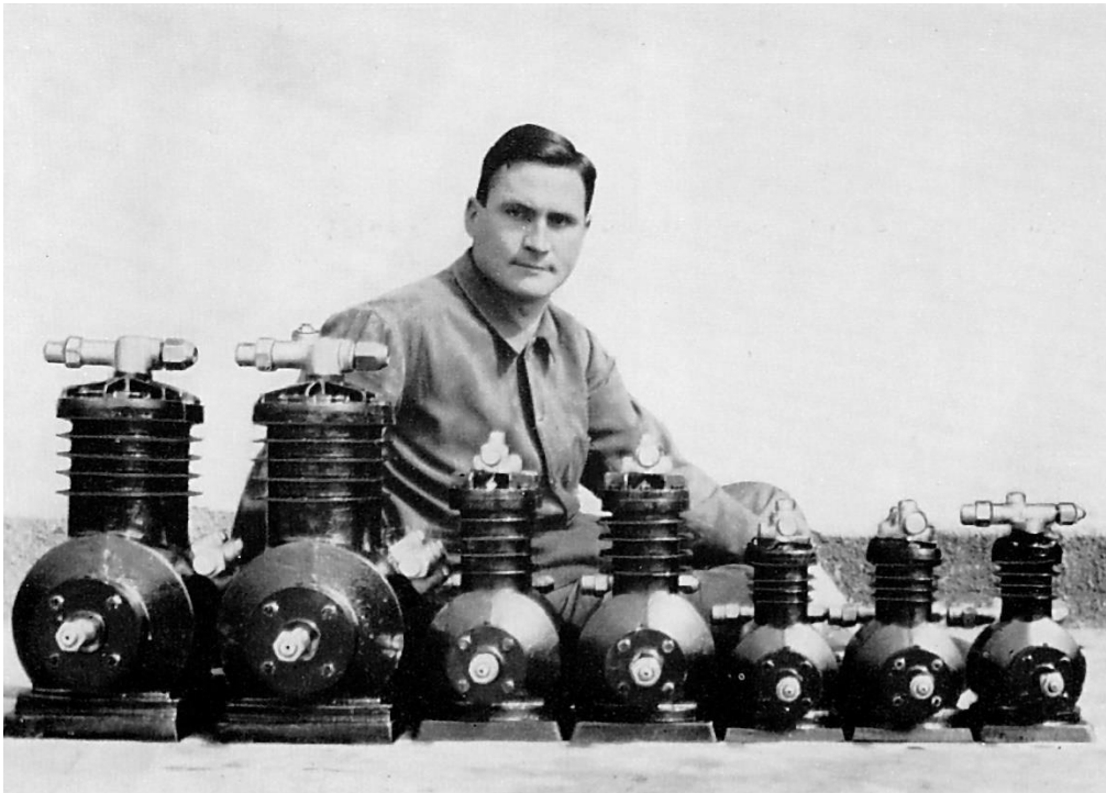
Image 2: Martin Bitzer started out manufacturing thermostatic expansion valves from steel, followed by compressors soon thereafter. The first BITZER compressors were reciprocating compressors with co-current flow design, shown here with Martin Bitzer in the background
