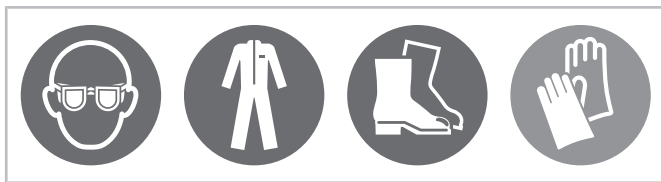
Fig. 2: Wear personal protective equipment!
