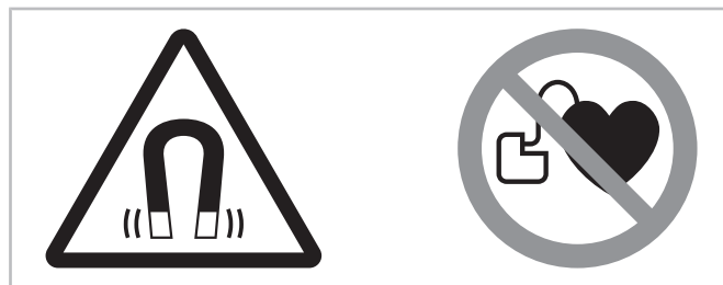
Fig. 8: Warning and prohibition signs on a compressor with permanent magnet motor
